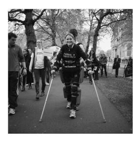
limbs and torso, giving her mobility through motion sensors, battery-operated motors and an onboard computer system.
